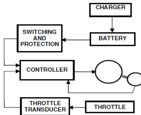
Figure 2. Electric propulsion system
