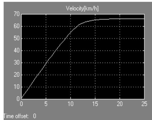
Figure 5. Simulation of vehicle acceleration at peak torque
