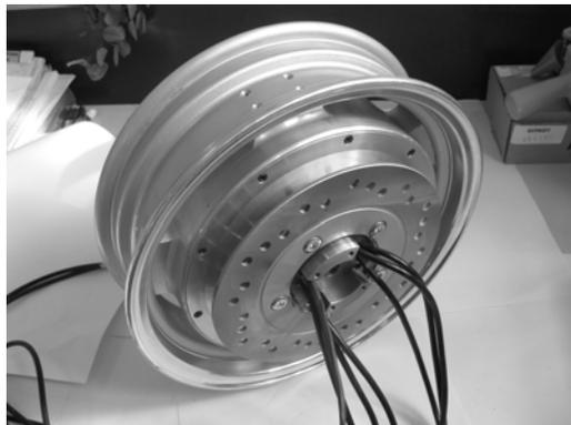
Figure 6. In-wheel "Brushless DC Motor
