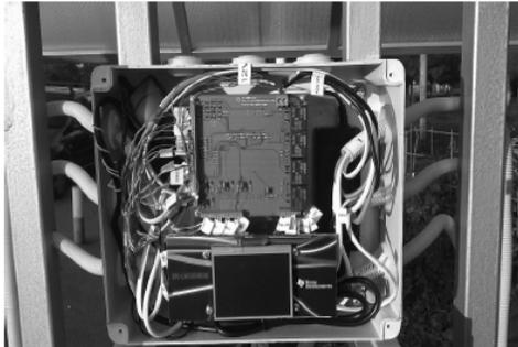
Figure 11. Station controller Stellaris and interface
