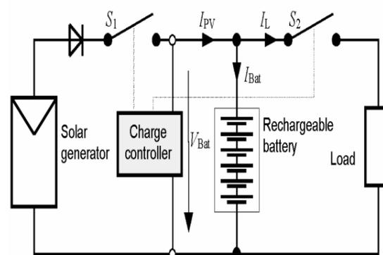
Figure 3. Technical connection scheme of the stand alone PV light system with a Led lamp
