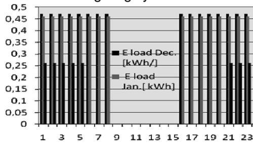
Figure 4. Load Pattern for a PV -street lamp
