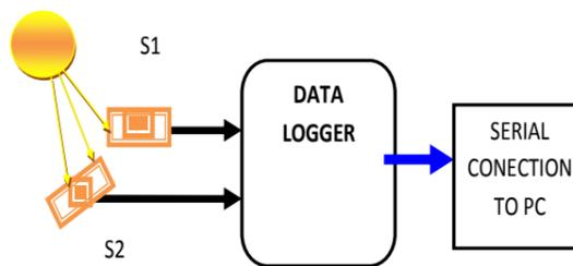
**Figure 2.** Structural scheme of the Solar radiation measurement unit
