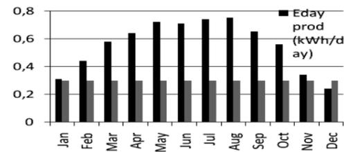
Figure 5. Comparison of daily loads, (kWh) and energy availability for lighting system.
