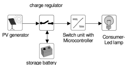
**Figure 1.** Principal structure of the photovoltaic street light system, (Source: Fraunhofer ISE, Freiburg, Germany).
