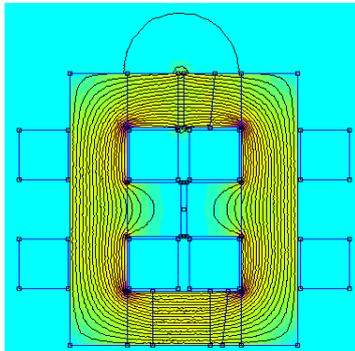
Figure 2.a). M.f.d. field lines in the device with the sample obtained with FEMM
