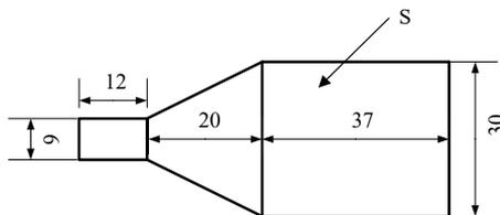
Figure 5.b). The field concentrator (top view)
