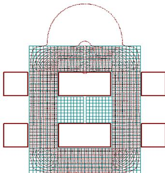
Figure 2.b). M.f.d. field lines in the device with the sample obtained with Green function method
