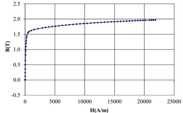
Figure 3. BH of the device's ferromagnetic material
