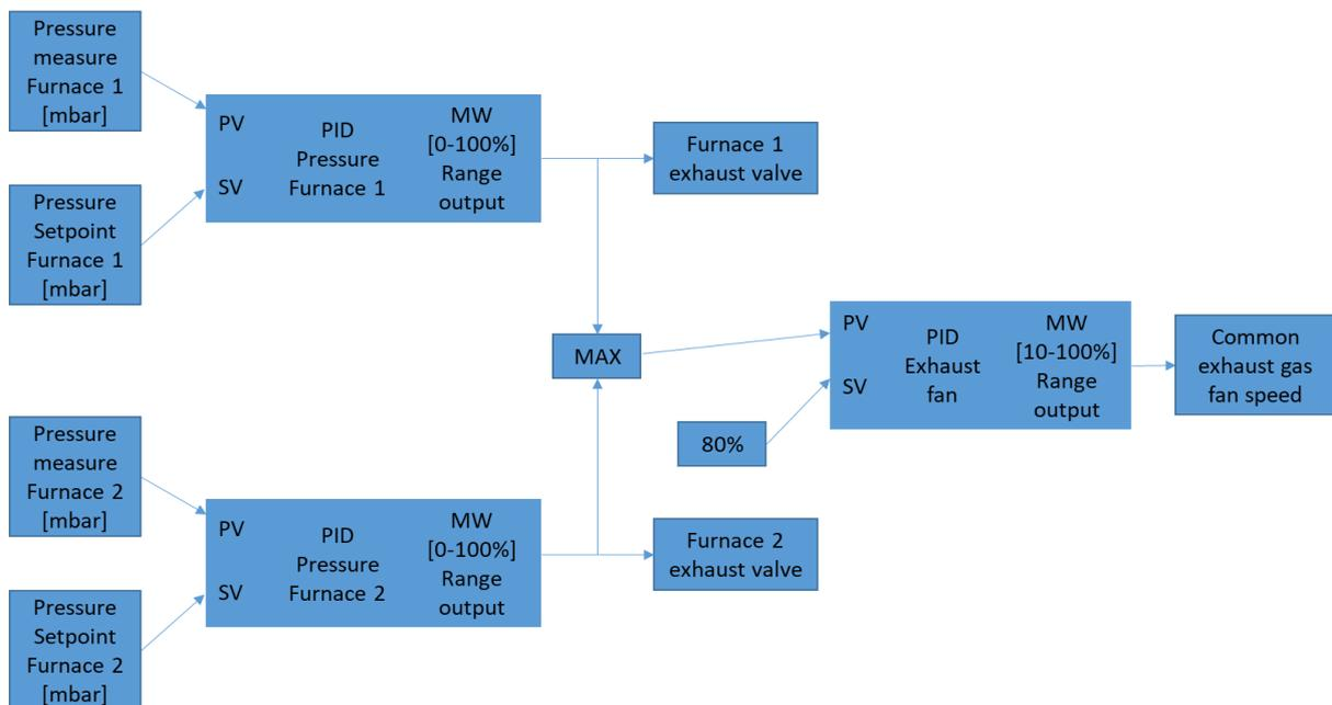
**Figure 5.** Logical diagram for controlling the inside pressure of both furnaces
