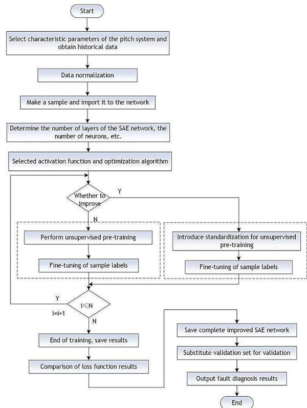
Figure 4. Fault diagnosis flowchart of wind turbine pitch system
