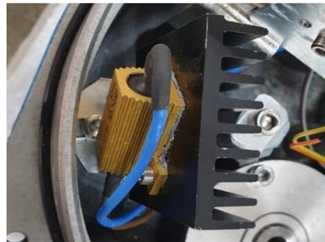
Figure 4. Anti-moisture resistor
