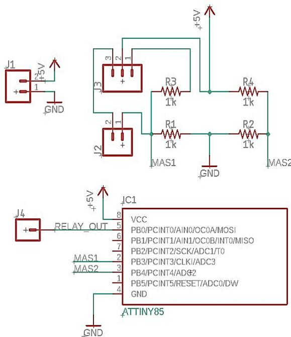
Figure 7. Microcontroller based thermostat
