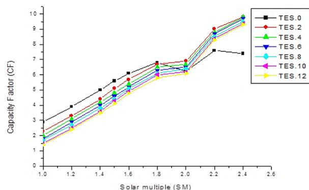
**Figure 7.** Multiple solar effect on the capacity factor (CF) under different solar TES values in the Bechar region, Algeria
