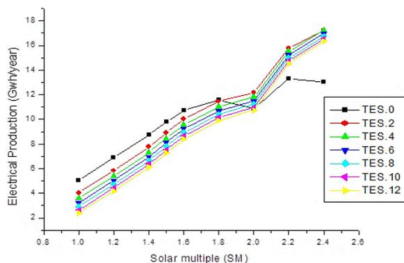
**Figure 6.** Multiple solar effect (SM) on electricity production under different solar TES values in the Bechar region, Algeria
