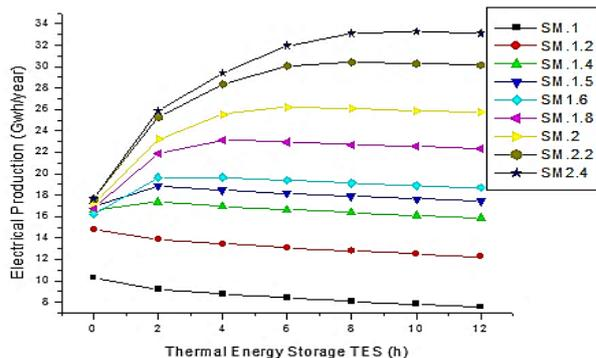
**Figure 2.** Effect of TES on the production of electricity under different values of solar multiple in the region of Djelfa, Algeria
