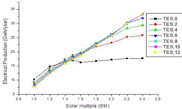
**Figure 3.** Multiple solar effect (SM) on electricity production under different TES values in the Djelfa region, Algeria
