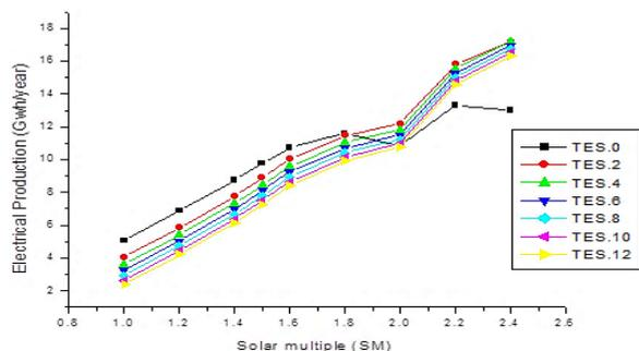
**Figure 4.** Multiple solar effect on the capacity factor (CF) under different TES values in the Djelfa region, Algeria
