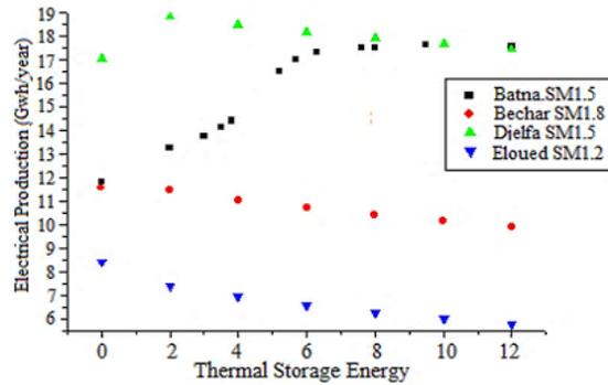
**Figure 9.** Effect of TES on electricity production in different regions in Algeria with optimal SM values
