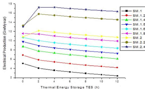
**Figure 5.** Effect of TES on electricity production under different values of solar multiple in the Bechar region, Algeria
