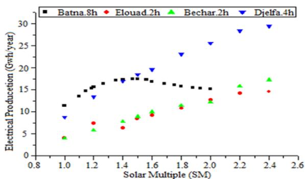
**Figure 10.** Multiple solar effect (SM) on electricity production in different regions in Algeria with the optimal values of TES
