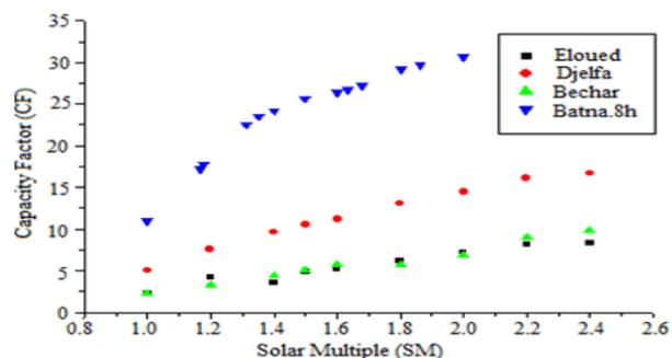
**Figure 11.** Multiple solar effect on the capacity factor CF in different regions in Algeria with the optimal values of TES
