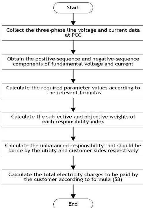
Figure 7. The flowchart of realizing the new adjustment scheme of electricity charges
