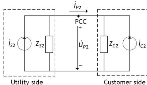
Figure 2. Negative-sequence equivalent circuit
