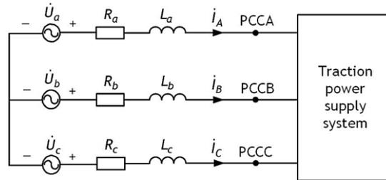
Figure 8. Simulation model
