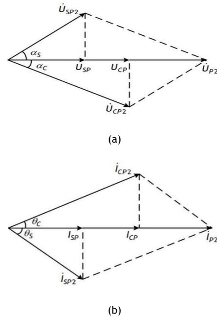
Figure 3. Negative-sequence voltage and current phasor diagram
