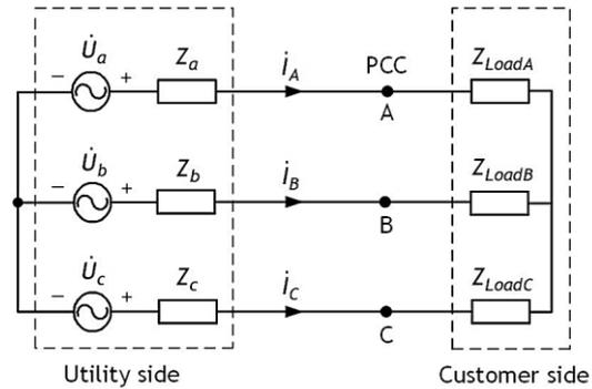
Figure 1. Schematic diagram of the three-phase three-wire power system
