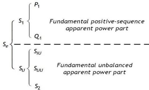
Figure 5. The decomposition of the equivalent apparent power
