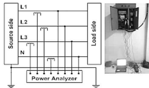
Figure 1. Electric parameter measurements using a power analyser
