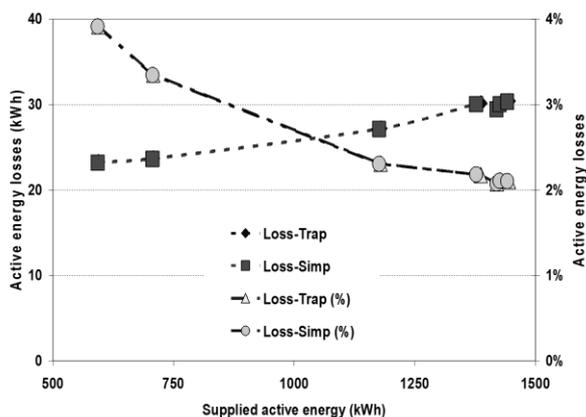
Figure 5. Energy losses versus supplied energy
