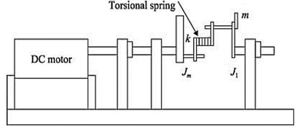
Figure 1. Manipulator arm actuated by DC motor
