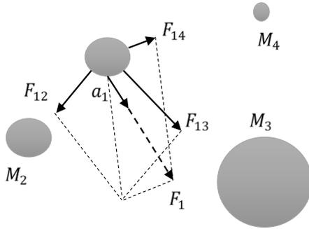
Figure 3. Acceleration and force vector
