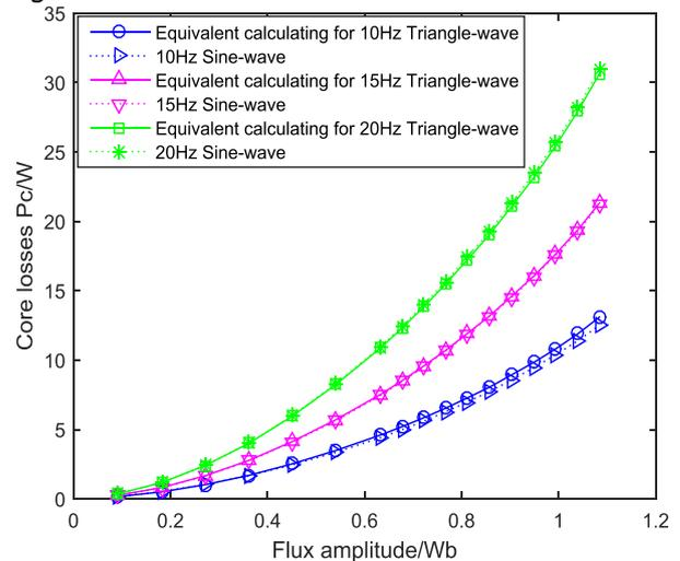
**Figure 6.** Comparisons of the losses of sine wave and the converted core losses of triangular wave at the same frequency without considering excess loss
