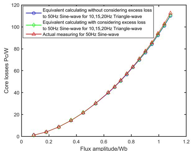
**Figure 7.** Comparisons of the converted core losses of triangular wave from 10,15,20 Hz to 50 Hz and those of the measured sine wave at 50 Hz considering excess loss and without considering excess loss
