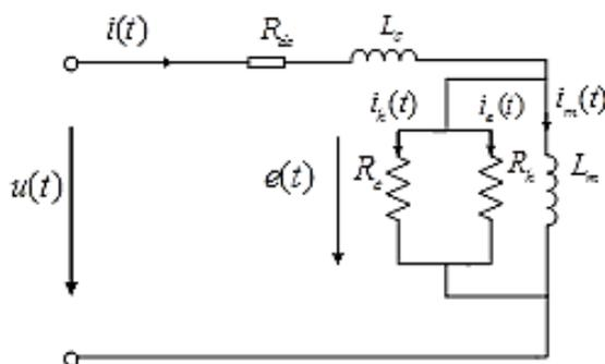
Figure 1. No-load circuit model of single-phase transformer
