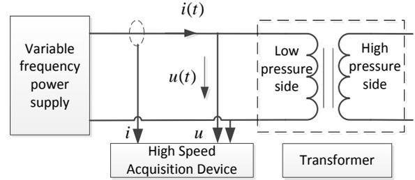
Figure 2. The schematic diagram of the experimental device
