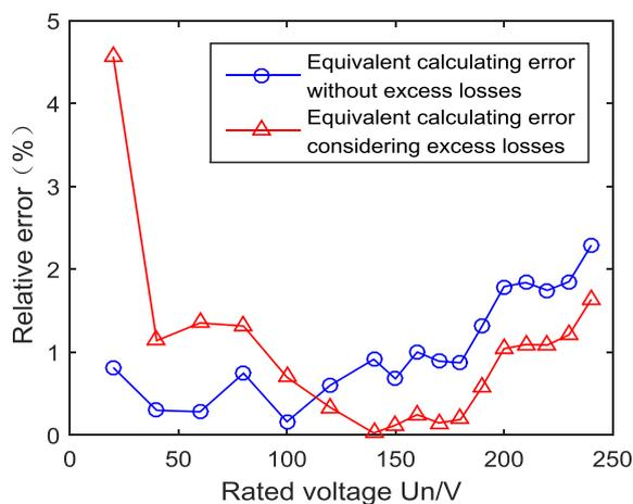
Figure 8. Comparisons of the relative error curves of the converted core losses for triangular wave from 10,15,20 Hz to 50 Hz considering excess loss and without considering excess loss
