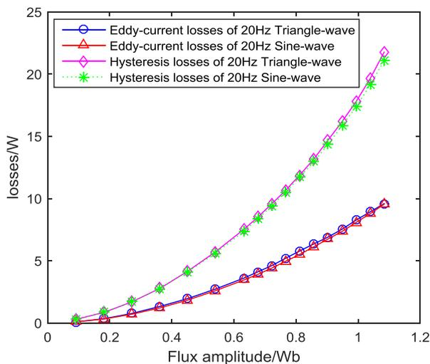
**Figure 5.** Comparisons of the core losses components of sine wave and triangular wave at the same frequency without considering excess loss
