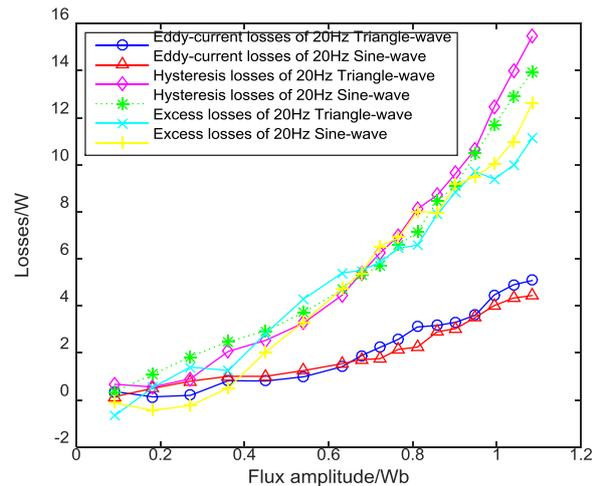
**Figure 3.** Comparisons of the core loss components of the same frequency sine wave and triangular wave considering excess loss
