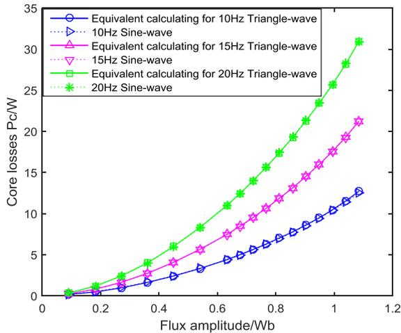
**Figure 4.** Comparisons of the core losses of sine wave and the converted that of triangular wave at the same frequency considering excess loss
