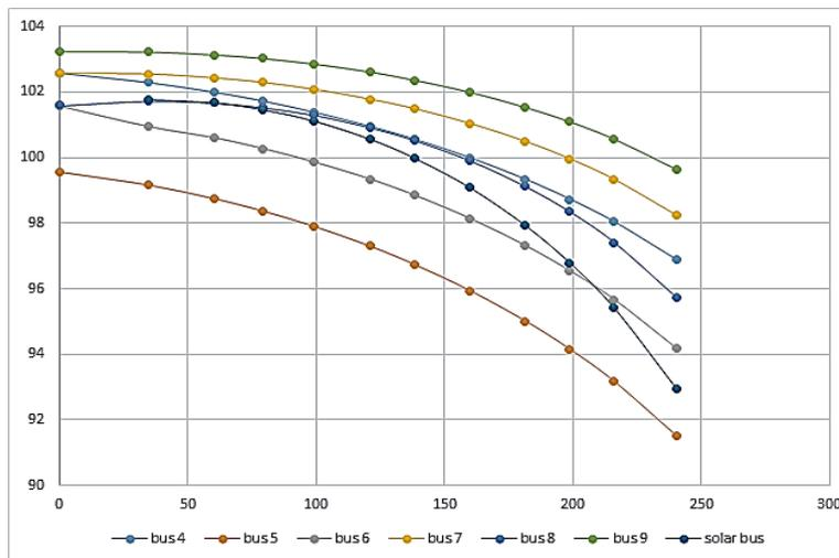
Figure 5. Voltage profiles for IEEE 9-Bus system containing solar bus at Bus 8 (case 3)
