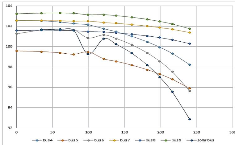
Figure 4. Voltage profiles for IEEE 9-Bus system containing solar bus at Bus 6 (case 2)
