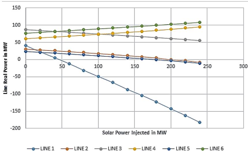
Figure 7. Plot of real power in transmission lines at various solar PV penetration levels
