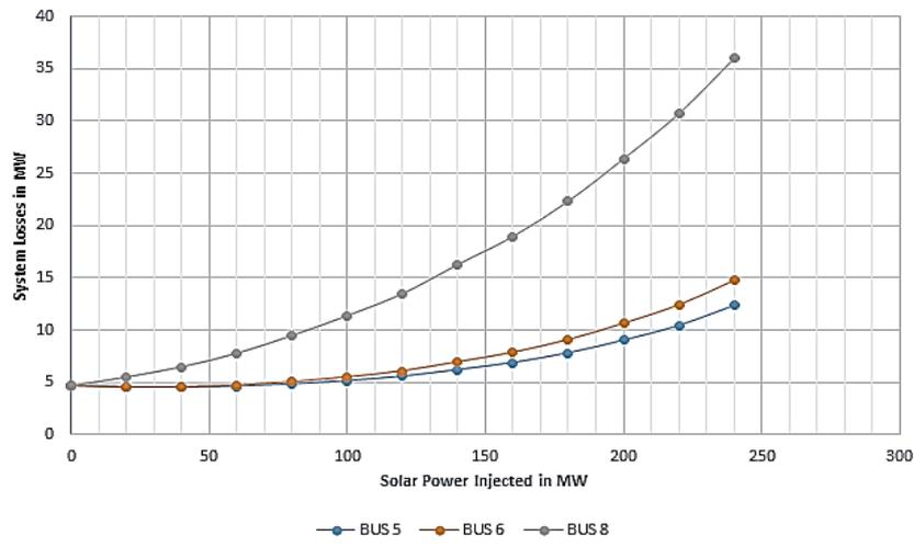
Figure 6. Plot of system losses in MW v/s solar penetration levels for injection at various bus locations
