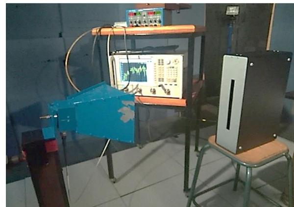
Figure 2. Measuring bench in semi-anechoic room
