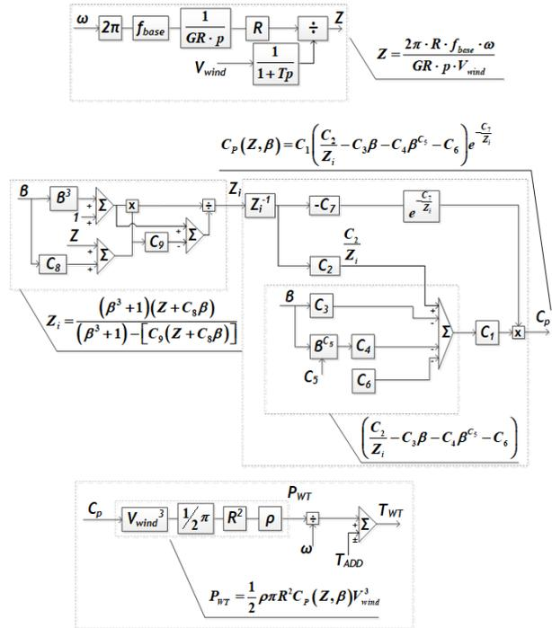
Figure 2. Schematic structure of the WT mathematical model:  $GR$  - gear ratio;  $p$  - electric machine pole pairs;  $T_{ADD}$  - additional mechanical torque for different tests;  $T_{WT}$  - resulting mechanical torque of WT;  $f_{base}$  - network frequency
