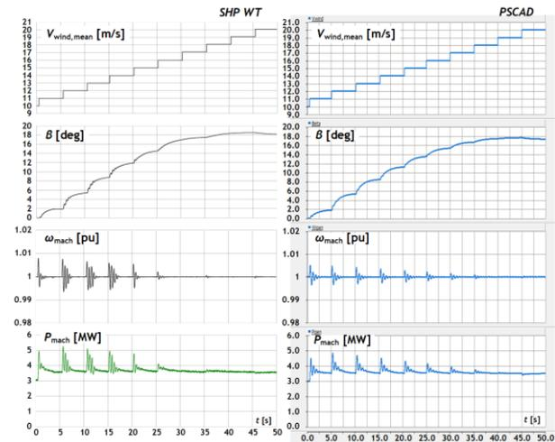
Figure 6. Resulting oscillograms of the operation of the WT pitch control in case of steps in wind speed (from 10 m/s up to 20 m/s)
