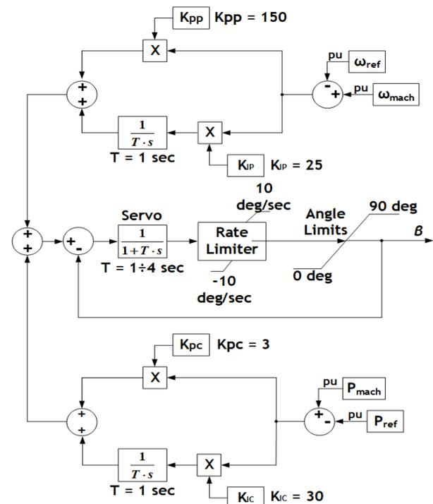
Figure 3. Schematic structure of pitch control model:  $K_{pp}$  - proportional frequency coefficient;  $K_{ip}$  - integral frequency coefficient;  $\omega_{ref}$  - WT shaft rated speed;  $\omega_{mach}$  - current WT shaft speed; Servo - servomotor;  $K_{pc}$  - proportional active power coefficient;  $K_{ic}$  - integral active power coefficient;  $P_{ref}$  - WT rated active power;  $P_{mach}$  - current WT active power
