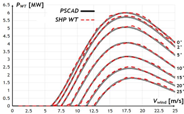
Figure 5.  $P_{WT} = f(V_{wind})$  curves for Case 2
