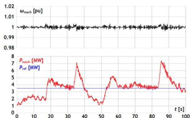
Figure 7. Resulting oscillograms of the operation of the WT pitch control in case of wind dynamic model
