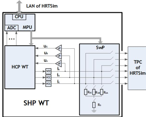
**Figure 1.** SHP WT schematic structure: LAN - local area network; CPU - central processing unit; ADC - analogue-to-digital converter; MPU - microprocessor unit; HCP WT - hybrid coprocessor of WT; VCC - voltage-current converter; VF - voltage follower; SwP - switching processor; TPC - three-phase commutator cross-board; RG, RGA, RGB, RGC - ground fault resistance; U<sub>a</sub>, U<sub>b</sub>, U<sub>c</sub> - voltage; i<sub>a</sub>, i<sub>b</sub>, i<sub>c</sub> - current
