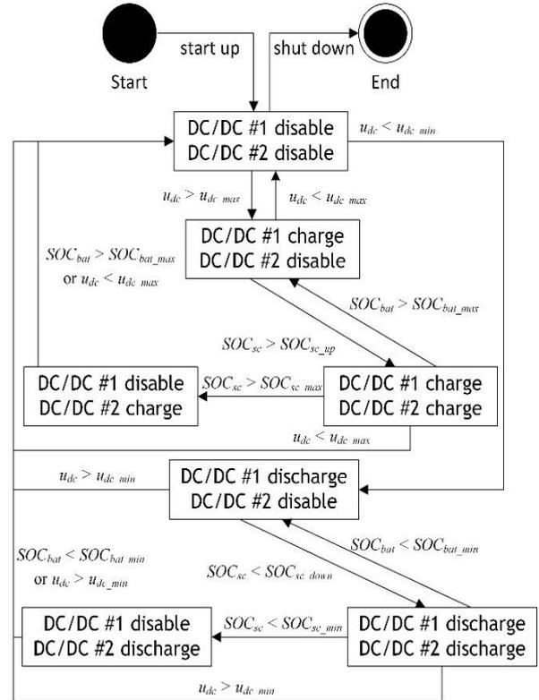
Figure 3. State machine of HESD's energy control
