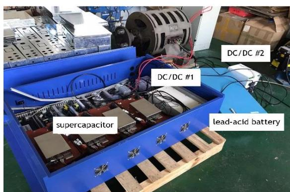
Figure 5. Hybrid energy storage device
