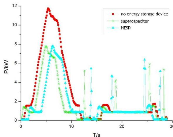
Figure 7. Power consumptions of no ESD, supercapacitor and HESD
