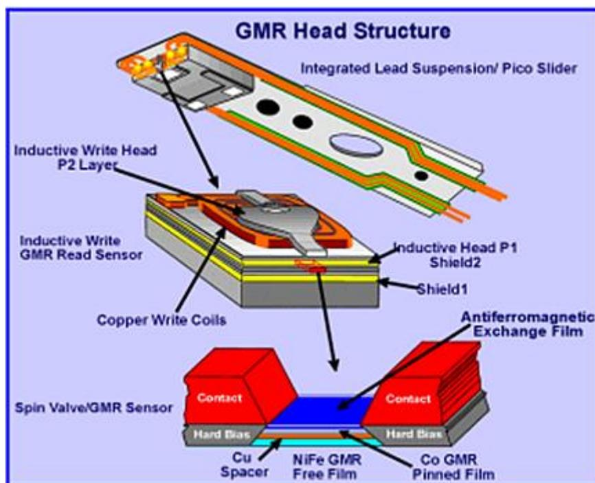
Figure 2. Commercial IBM giant magnetoresistance read head [9]
