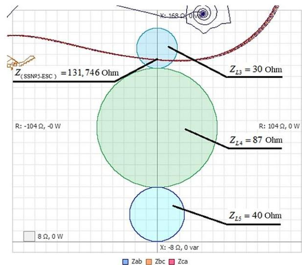
Figure 7. Resistance locus when OSP is checked in the network when STATCOM is connected to SS №5 buses
