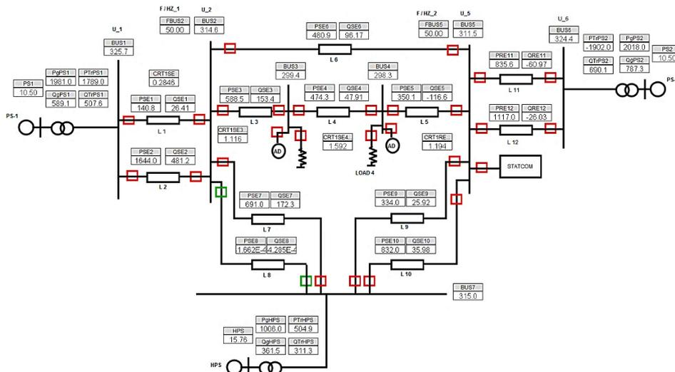
Figure 3. Scheme with STATCOM connected to buses of SS №5.
