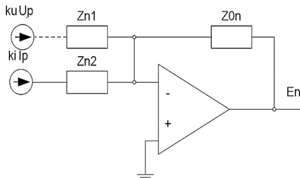
Figure 1. Equivalent scheme for the formation of the n-th compared value
