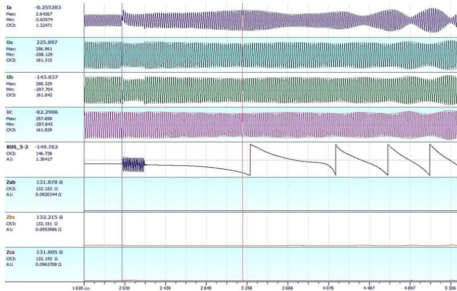
Figure 5. Oscillograms of phase A current, voltages of three phases, angle, resistances in asynchronous mode with STATCOM connected to SS №5 buses
