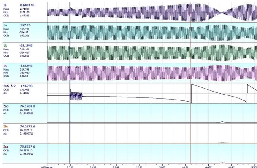
Figure 4. Oscillograms of current phase A, voltages of three phases, angle, resistance in asynchronous mode without connecting STATCOM
