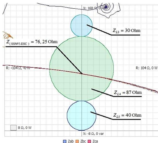
Figure 6. Resistance locus when OSP is checked in the network without connecting STATCOM
