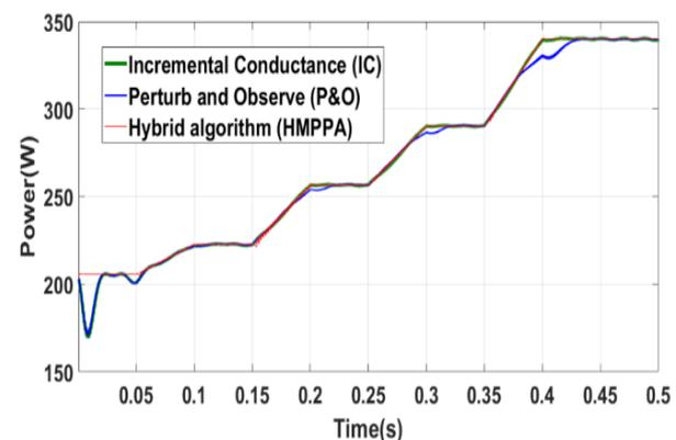
Figure 5. Response of three algorithms (IC, P&O, HMPPA) under gradual change of the irradiance
