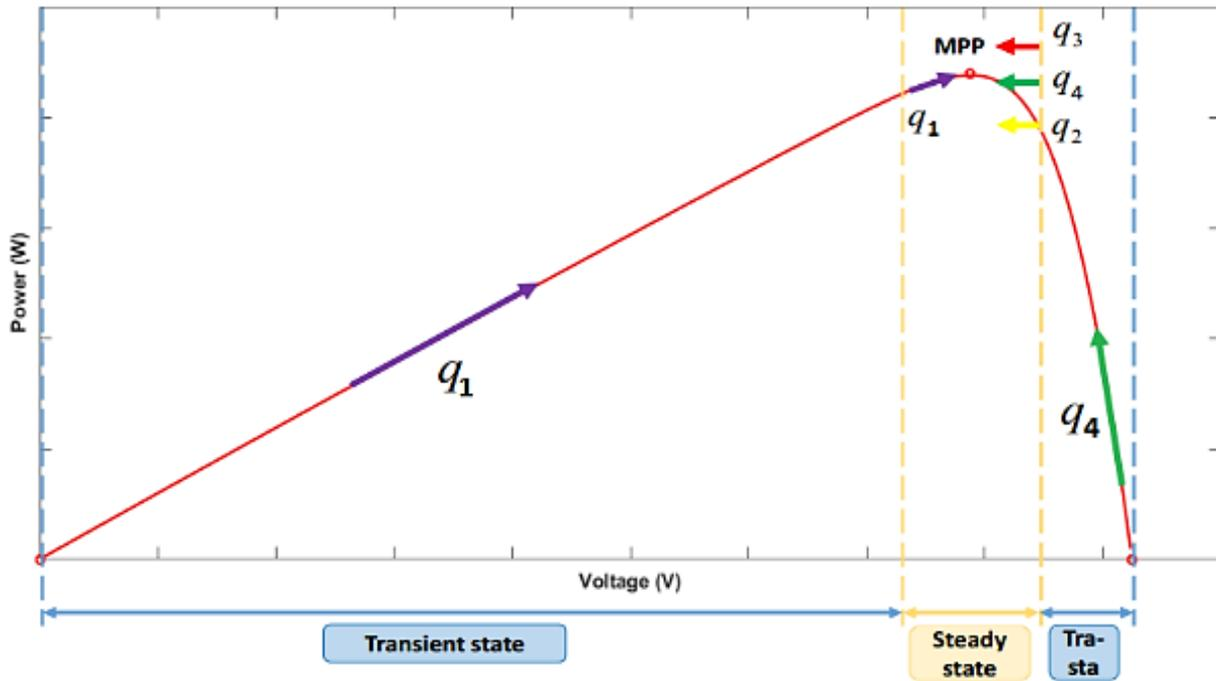
Figure 2. Evolution of the MPP tracking in the P-V curve
