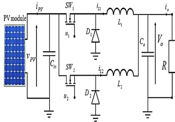
Figure 1. Structure of the photovoltaic module with 2-phase interleaved buck converter (PV-2IBC)
