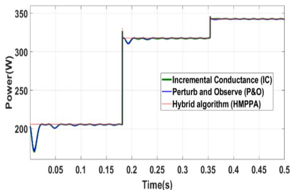
Figure 6. Response of three algorithms (IC, P&O, HMPPA) under step change of the irradiance
