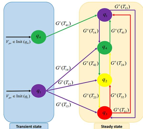
Figure 3. The proposed hybrid automaton of the photovoltaic system (PV-2IBC)
