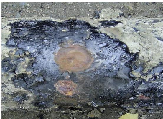
Figure 1. Typical image of corrosion by DC stray currents
