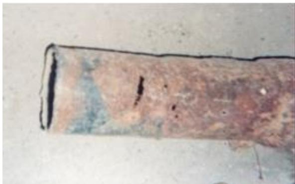
**Figure 2.** Underground gas pipelines with degraded insulation and corrosion generalized by the action of AC stray currents and pierced in the form of funnel by the DC stray currents
