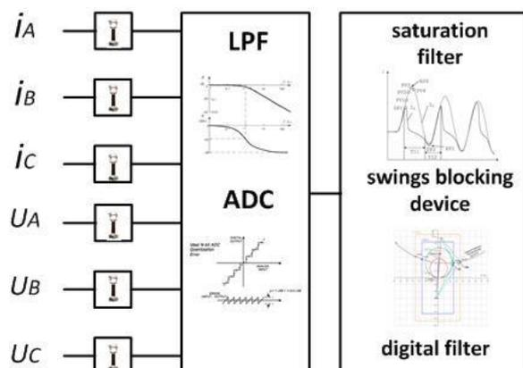
Figure 1. A block diagram of a relay protection device
