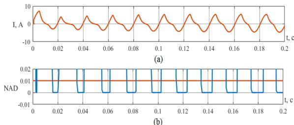
Figure 2. (a) Secondary current of saturated CT; (b) NAD signal and level of comparison 0.01
