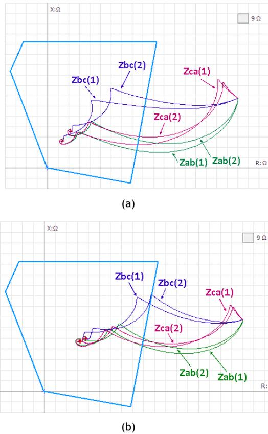
Figure 3. Near (a) and far (b) reservations: hereinafter, the index (1) is a simplified model of DP, (2) is a detail model of DP
