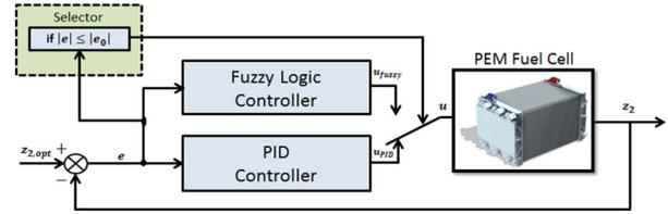
Figure 6. Structure of the hybrid Fuzzy-PID controller
