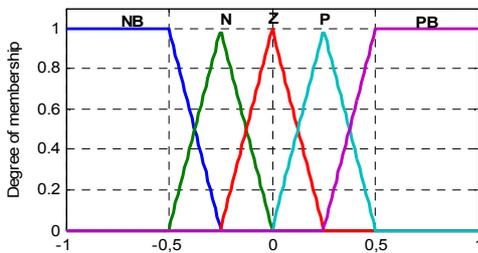
Figure 4. Membership functions of inputs ( $e, \Delta e$ )
