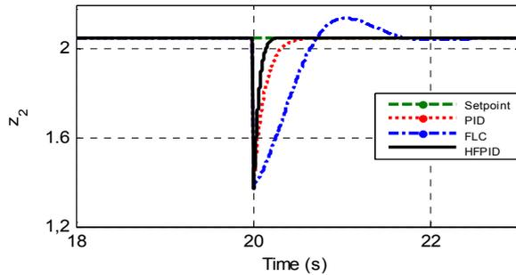
Figure 9. The magnified plot of oxygen excess ratio variation at  $t=20$ s
