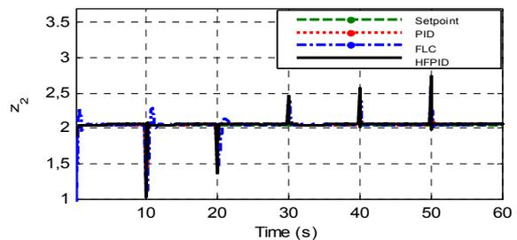
Figure 8. Response of oxygen excess ratio for different control strategies
