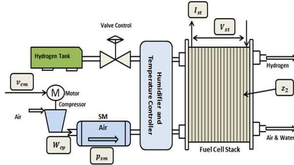
Figure 1. Fuel Cell System showing control inputs and outputs
