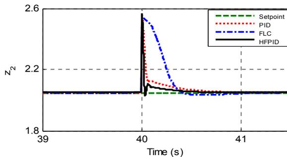
Figure 10. The magnified plot of oxygen excess ratio variation at  $t=40$  s
