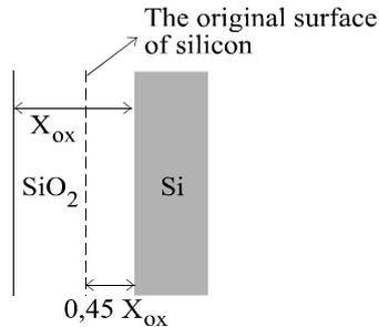
Figure 5.2. The oxide layer grows by the consumption of a silicon layer (adapted after Bârsan [16])
