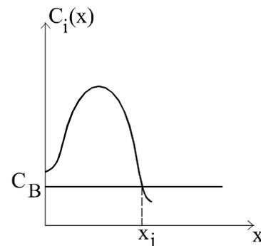
Figure 5.14. The junction formation in the case of shallow ion implantation
