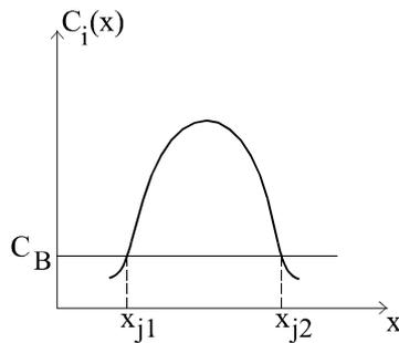
Figure 5.15. The junction formation in the case of deep ion implantation
