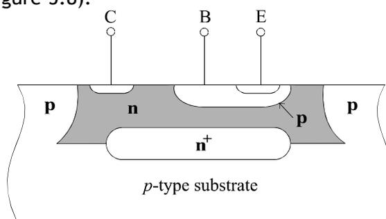
Figure 5.8. Section through the structure of a bipolar transistor made in an epitaxial layer (adapted after Gray and Meyer [15])
