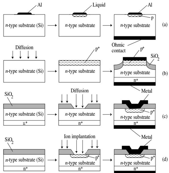
**Figure 5.1.** Technologies for the execution of the pn junction: (a) alloyed junction; (b) diffused junction; (c) planar junction; (d) planar junction obtained by ion implantation (adapted after Sze [10])
