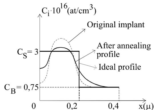
Figure 5.17. The profile of the implanted impurities below the oxide layer of the gate. The ideal profile is used to estimate the threshold voltage variation obtained by ion implantation (adapted after Wolf [19])
