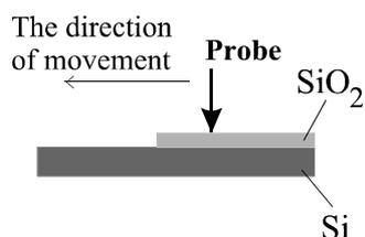
Figure 5.6. Profilometer method for measuring the thickness of the oxide layer
