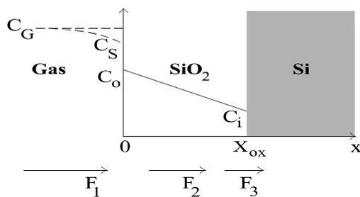
Figure 5.3. Model for thermal oxidation of silicon (adapted after Bârsan [16])
