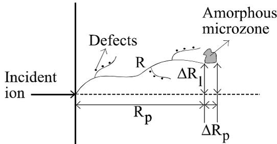
Figure 5.13. The trajectory of the implanted ions in a solid target (adapted after Barsan [16])
