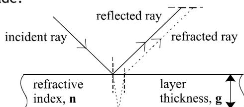
Figure 5.7. The principle of optical interference on the blade parallel plane faces to measure the thickness of the oxide layer
