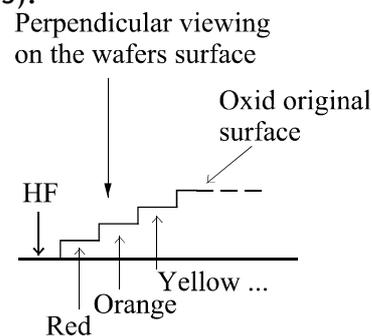
Figure 5.5. The HF drop method for measuring the thickness of the oxide layer
