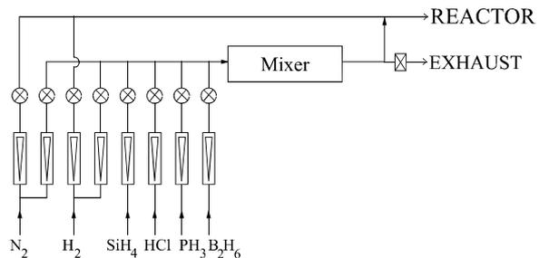
Figure 5.10. The scheme of the gas distributor
