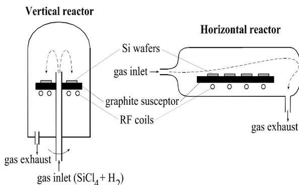
Figure 5.9. The scheme of the horizontal and vertical reactors for the epitaxial growth
