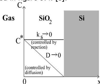
Figure 5.4. Distribution of oxidizing species in the oxide layer for the two limit cases oxidation model (adapted after Grove [8])
