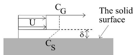
Figure 5.12. The stationary layer model (adapted after Grove [8])
