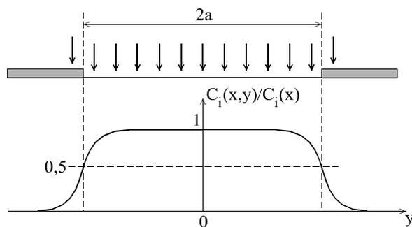
Figure 5.16. Side profile of impurities implanted through a  $2a$  window width and infinite length (adapted after Barsan [16])
