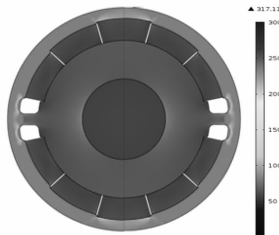
Figure 9. Von Mises stress distribution (MPa) in final version of rotor with buried magnets
