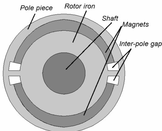
Figure 7. Initial structure of rotor with buried magnets
