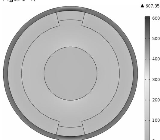
Figure 4. Von Mises stress distribution (MPa) in the first rotor
