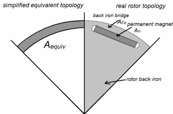
Figure 3. Simplified assumption of a rotor with buried magnets
