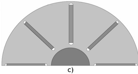
Figure 1. Rotor configuration for high-speed PMSM: a) Surface-mounted magnets; b) Buried magnets; c) Buried magnets with flux concentration.
