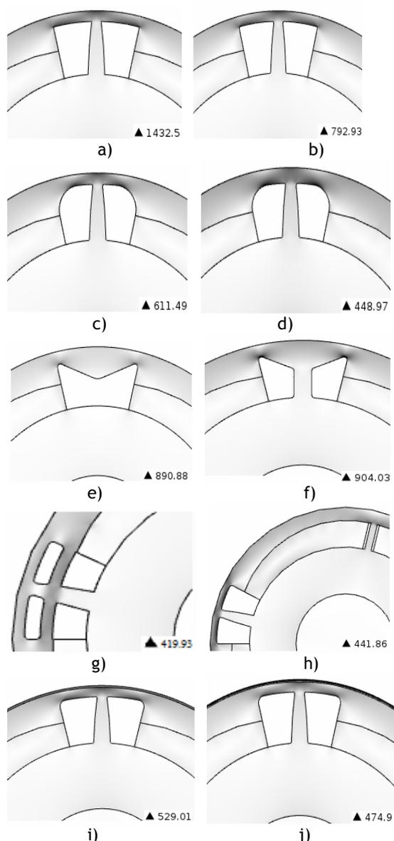
Figure 8. Various shape and dimensions of the pole piece bridges
