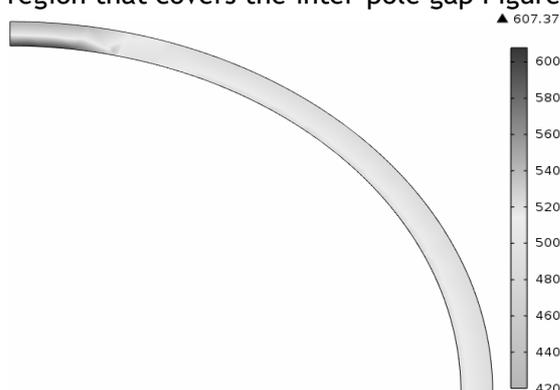
Figure 5. Mechanical stress concentration (MPa) on the retainer ring
