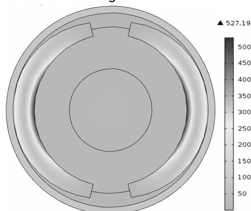
Figure 6. Von Mises stress distribution (MPa) in the second rotor
