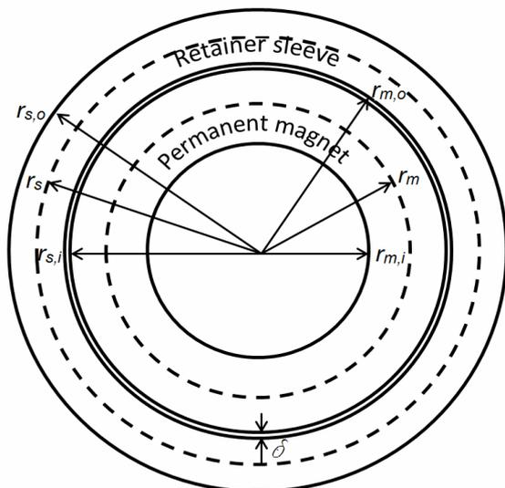
Figure 2. Geometry assumption of permanent magnet and retainer sleeve in a rotor with surface-mounted magnets
