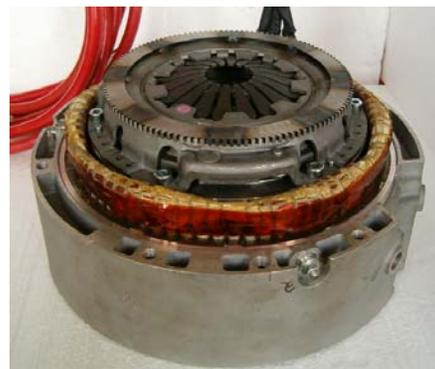
**Figure 14** Permanent magnets motor
